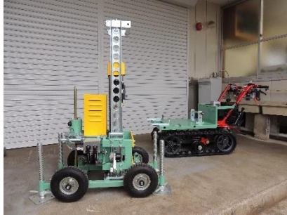
Converted to 4-wheel tire type survey machine
